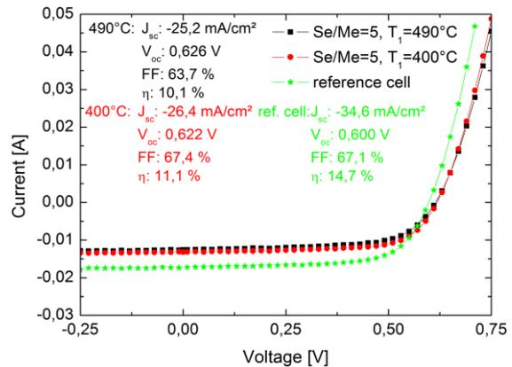
**Figure 5:** I-V curves from the best solar cells made from the Selenium variation in comparison to our reference solar cell.
