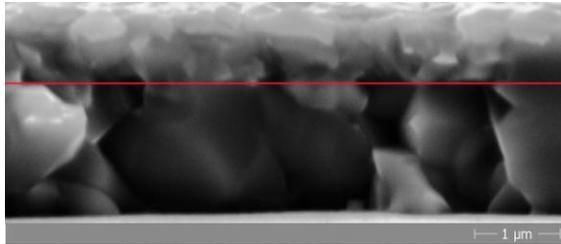
**Figure 4:** Cross-section view of the sample Se/Me=5 (400°C). The red line indicates the grain boundary at 1/3 film thickness.
