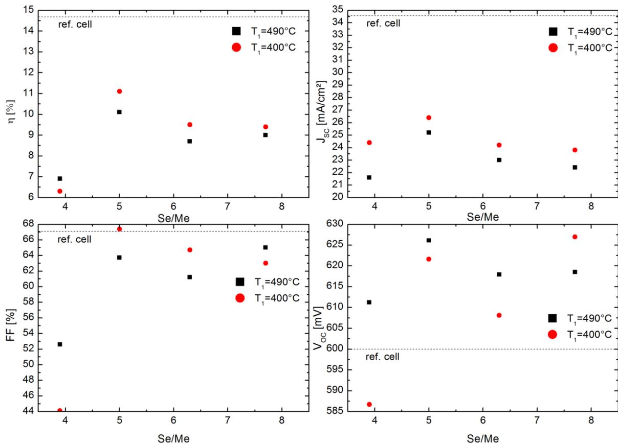
**Figure 6:** Solar cell parameters as a function of the Se/Me ratio. As comparison the parameters of the reference cell are represented by the dotted line.
