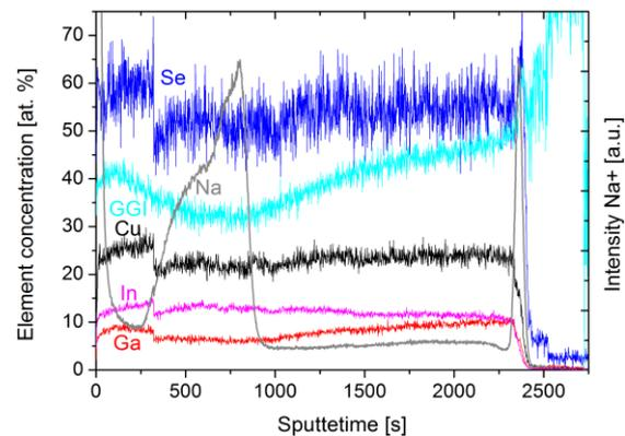
**Figure 3:** ToF-SIMS depth profile for 400°C first stage substrate temperature with  $\text{Se/Me}=7.7$ .
