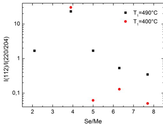
**Figure 2:** Intensity ratios  $I_{(112)}/I_{(220)/(204)}$  versus Selenium to Metal fluxes.
