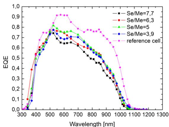
**Figure 7:** External quantum efficiency measurements for  $400^\circ\text{C}$  first stage substrate temperature with respect to the Se/Me-ratio.
