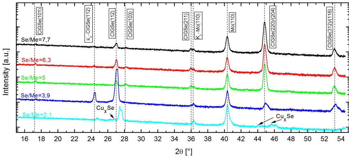
**Figure 1:** X-ray diffraction pattern for 400°C first stage temperature with different Se/Me-fluxes. The diffraction patterns for 490°C, show a similar behavior.
