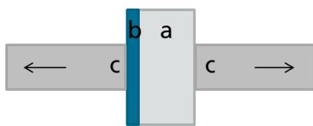
**Fig. 3, Pull test schematically, a glass, b CIGS, c metal cylinders glued on the sample surface, the arrows indicate the applied forces.**
