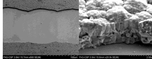
**Fig. 2, SEM micrographs of the P3 scribe edge. The left figure shows an overview of the scribe. The scribe edges and the bottom of the scribe nearby are free from molten CIGS or other residuals.**
