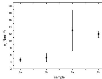
**Fig. 4, Adhesive stress from pull test measurements with samples of group 1 (1a, 1b) showing reduced adhesive forces in than to samples of group 2 (2a, 2b).**
