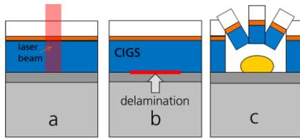
**Fig. 1, Laser scribing process schematically, step a: heating of CIGS, step b: delamination, step c: explosive lift-off process with molten CIGS residual (yellow)**
