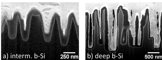
FIG. 2. SEM cross sections of the intermediate (a) and the deep (b) b-Si structure covered by thermal ALD deposited  $\text{Al}_2\text{O}_3$  (dark grey). The bright grey line is the Si- $\text{Al}_2\text{O}_3$ -interface. The structures were protected by Pt before cross-section preparation (white coating).
