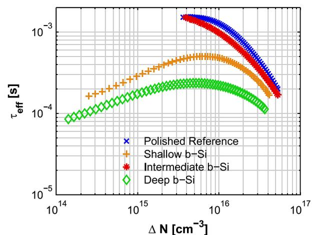
FIG. 3. Injection level dependent lifetime of the three model structures in comparison to a polished reference passivated with 100 nm of  $\text{Al}_2\text{O}_3$ . The samples were annealed in low pressure Ar ambient at  $425 \text{ }^\circ\text{C}$  for 30 min.
