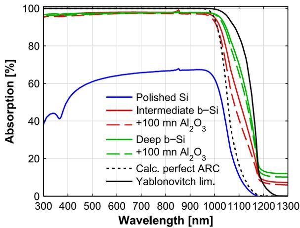
FIG. 1. Experimental absorption spectra of the intermediate (red) and deep (green) b-Si structures before (solid) and after (dashed) coating with 100 nm  $\text{Al}_2\text{O}_3$ . For comparison, the experimental absorption spectrum of a polished wafer (solid blue), as well as theoretical spectra of a perfect anti-reflection coating (dash-dotted black) and a perfect anti-reflection coating with Lambertian scattering (Yablonovitch limit, solid black) are also plotted.
