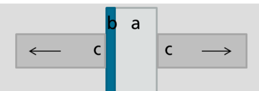
[Fig. 4] pull test (schematic view), a glass, b CIGS, c metal cylinders glued on the sample surface
