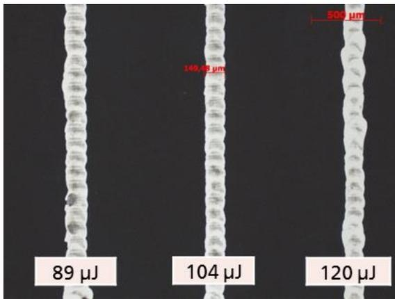
**Fig. 2, Optical micrograph of successfully ablated P3 laser scribes for different pulse energies. Residuals are visible in the scribe center.**
