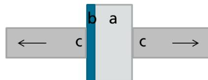
**Fig. 1, Pull test schematically, a glass, b CIGS, c metal cylinders glued on the sample surface, the arrows indicate the applied forces.**
