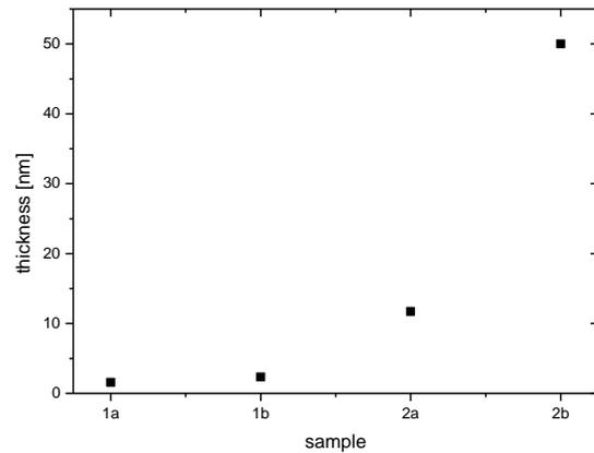
Fig. 8, thickness of the MoSe<sub>2</sub> layers, determined with TEM calibrated ToF-SIMS depth profiling (indicate the tolerances of the measurement).
