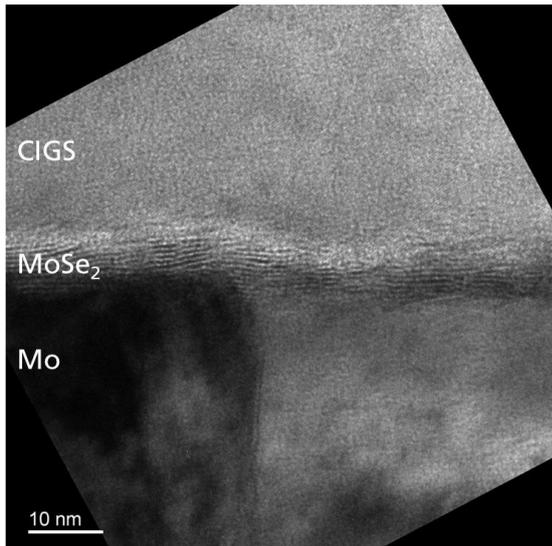
Fig. 6, TEM micrograph of MoSe<sub>2</sub> layer of the sample 2a, the MoSe<sub>2</sub> sheets are clearly visible. The orientation is mainly parallel to the Mo surface.
