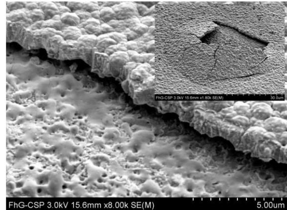
**Fig. 4, At the inset, a SEM micrographs of a small laser ablation structure (diameter 5  $\mu\text{m}$ ) is shown. The high resolution image displays a detail of the scribe edge and bottom. ZnO is removed selectively. The CIGS surface is molten and recrystallized close to the scribe edge. Some ZnO delamination is visible at the edge.**
