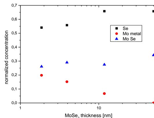
**Fig. 11, Mo (metallic, Se coordination) and Se surface concentration the Mo surface for different MoSe<sub>2</sub> thicknesses. The Mo metal peak vanishes for thicker MoSe<sub>2</sub> layers, due to the limited information depth of XPS.**
