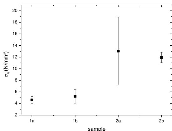
**Fig. 9, Adhesive stress from pull test measurements with samples of group 1 (1a, 1b) showing reduced adhesive forces in comparison to samples of group 2 (2a, 2b).**
