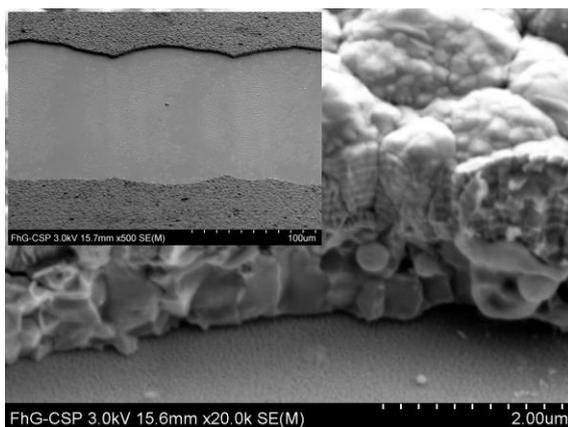
**Fig. 3, SEM micrographs of the P3 scribe edge. The inset shows an overview of the scribe. The scribe edges and the bottom of the scribe nearby are free from molten CIGS or other residuals.**
