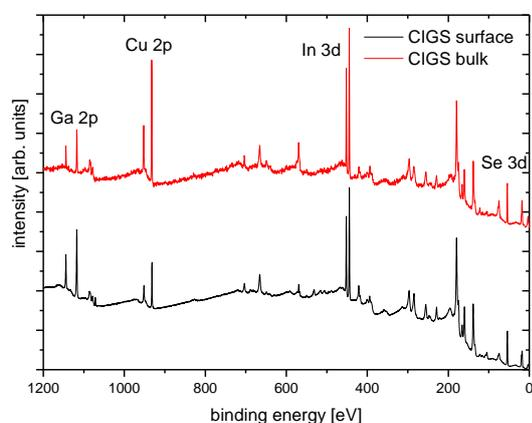
**Fig. 10 Composition of the delaminated CIGS surface from the Mo/CIGS interface (black curve) in comparison to CIGS bulk material (red curve) as measured by XPS**
