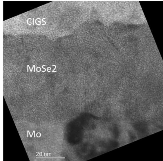
Fig. 7, TEM micrograph of MoSe<sub>2</sub> layer of the sample 2b, the MoSe<sub>2</sub> thickness is about 50 nm. The MoSe<sub>2</sub> sheets are not oriented in a preferred direction.
