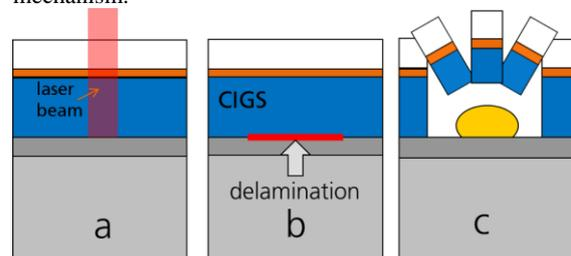
**Fig. 5, Laser scribing process schematically, step a: heating of CIGS, step b: delamination, step c: explosive lift-off process with molten CIGS residual (yellow)**
