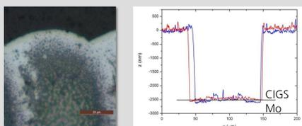
[Fig. 2] process successful, no melting at the scribe edge but some residuals on the scribe bottom
