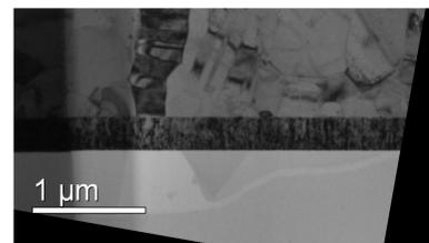
[Fig. 6] crosssection of the CIGS/Mo layer stack
