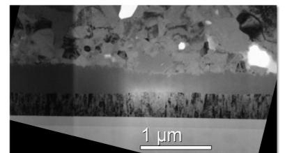
[Fig. 7] cross section of CIGS/MoSe<sub>2</sub>/Mo layer stack
