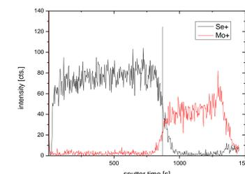
[Fig. 8] ToF-SIMS depth profile, an MoSe<sub>2</sub> layer is not visible
