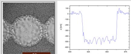
[Fig. 4] melting of the CIGS-Layer, Process was not successful
