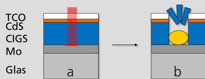
[Fig. 1] ns scribe process schematically, a) energy deposition at CIGS/Mo interface, b) explosive lift off
