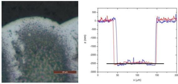
**Fig. 3**, process successful, no melting at the scribe edge but some residuals on the scribe bottom, profilometry shows sharp and vertical scribe edges
