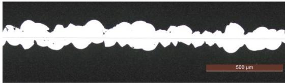
**Fig. 1,** mechanically applied scribe with area loss due to chipping
