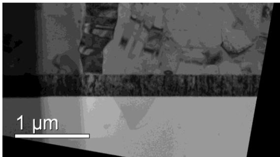
**Fig. 5**, crosssection of the CIGS/Mo layer stack
