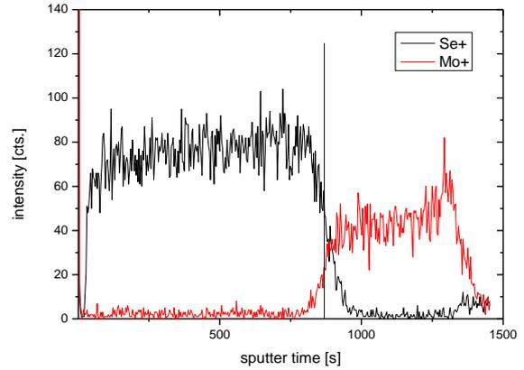
**Fig. 6**, ToF-SIMS depth profile, an MoSe<sub>2</sub> layer is not visible
