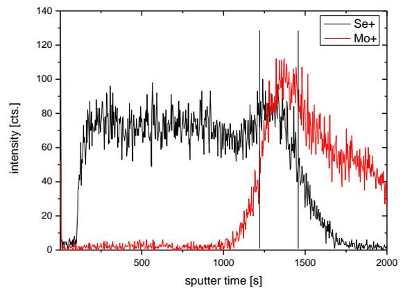
**Fig. 8**, ToF-SIMS depth profile, an MoSe<sub>2</sub> layer is visible
