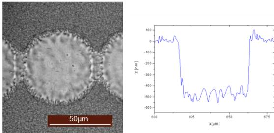
**Fig. 4**, melting of the CIGS-Layer, process was not successful, profilometry shows that the CIGS was not ablated completely (layer thickness 1,5 μm)
